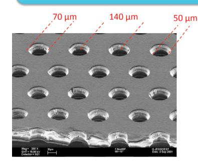
A Gas Electron Multiplier (F.Sauli, NIM A386 531 1997) is made of 50 µm thick kapton foil, copper clad on each side and perforated by an high surface-density of bi-conical channels.
